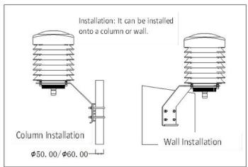
■ RJ45 interface PM2.5/PM10, TVOC, CO, T&RH Overall Size: width 190.00mm, height: 458.00mm
