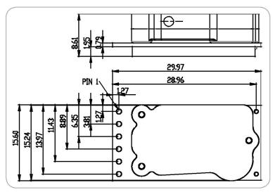
All dimensions in millimeters (mm)
