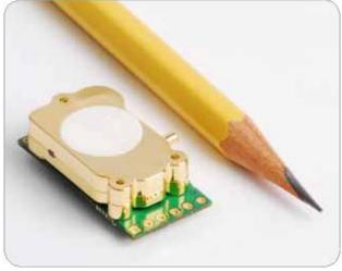
The Telaire<sup>®</sup> T6713 CO<sub>2</sub> Series is ideal for applications where CO<sub>2</sub> levels need to be measured and controlled for indoor air quality and energy saving applications such as demand control ventilation.
